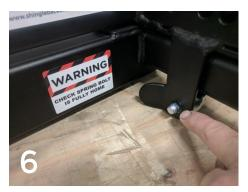
Make sure the spring bolt is fully home when closed, then clamp tight with the heavyduty clamp. The clamp should be firm to clamp shut. If it becomes loose it can be tightened with the U bolt nuts.
