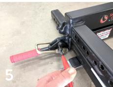
Fit the heavy duty clamp handle as shown making sure the circlip is seated in its groove.
