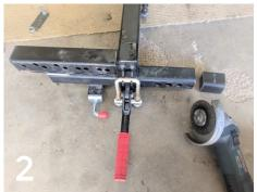
The swing arm comes with a long tow bar tube section to fit a wide variety of cars — in some instances, depending on your car, you *may* be required to trim a bit off the tube section to achieve the best fit for your car.
